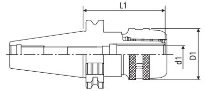
T.I.R.  $\geq 10\mu\text{m}/2.5xD$  Bal./rpm G6.3/10.000RPM
